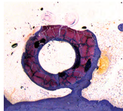
MAGNEZIX® CS conversion into calcium phosphate after 12 months with clear evidence of bone ingrowth.
